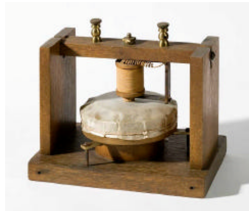
Replica of Bell's first telephone.
