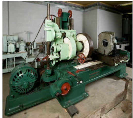
Richards universal facing, boring, drilling and milling machine.
