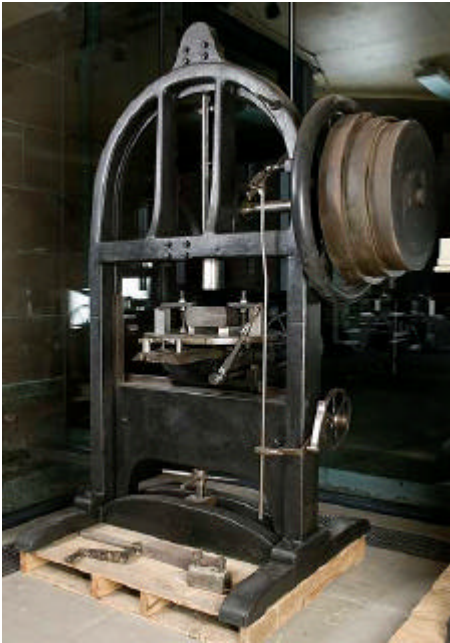
Sharp Roberts slotting machine, 1835 – the Museum's oldest machine tool.
